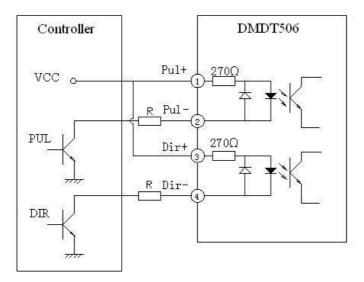
VCC=5V R=0 VCC=12V, R=1K $\Omega$  ( $\geq$ 1/8W) VCC=24V, R=2K $\Omega$  ( $\geq$ 1/8W)
