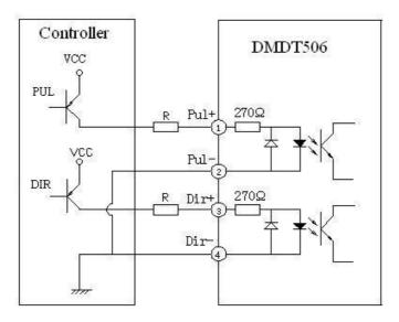
VCC=5V R=0 VCC=12V, R=1K $\Omega$  ( $\geq$ 1/8W) VCC=24V, R=2K $\Omega$  ( $\geq$ 1/8W)
